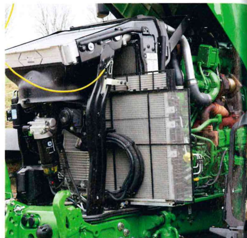
The 6250R gets the familiar 6.8-litre DPS motor but a bigger cooling pack. Test output and fuel use were excellent. Photos ST, HW.
