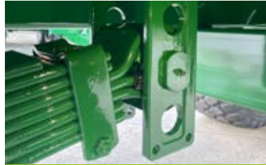
SPRUNG DRAWBAR ADJUSTMENT
