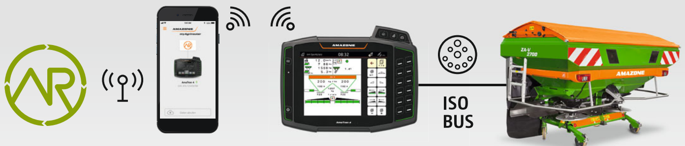
AMAZONE implements the connection to the ISOBUS machinery via the AmaTron 4
