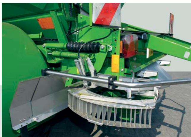
Limiter border spreading system in working position
