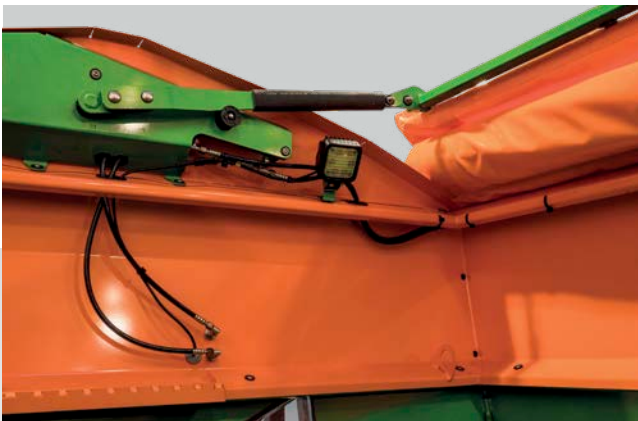
Work lights inside the hopper
