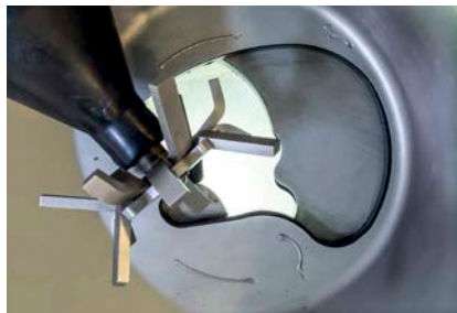
Stage 2: Hopper aperture half open
