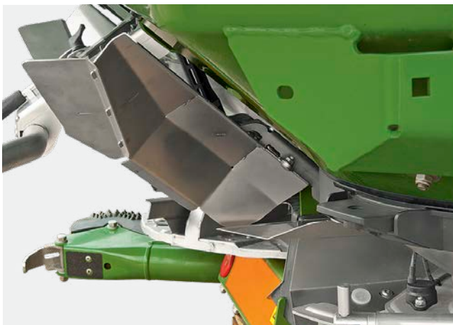
Border spread deflector swivelled upwards
