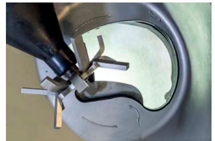
Stage 3: Hopper aperture wide open
