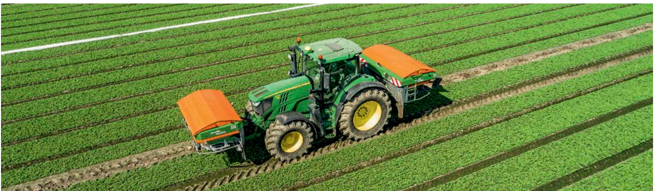
Precise spreading of two different fertiliser types
