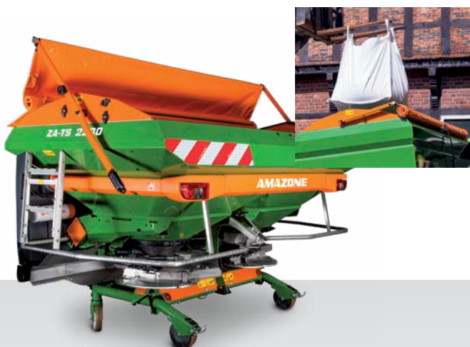
Swivel hopper cover, in its maintenance position for a simpler internal cleaning
