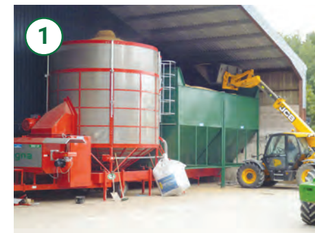
1 A 29 ton automatic dryer with a matched 29 ton wet grain hopper is loaded with wet grain stored inside the shed behind.
