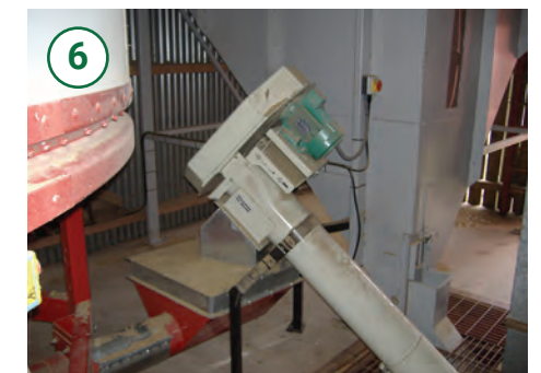
6 A bespoke intake hopper allows a dryer to be integrated into an existing grain handling system.
