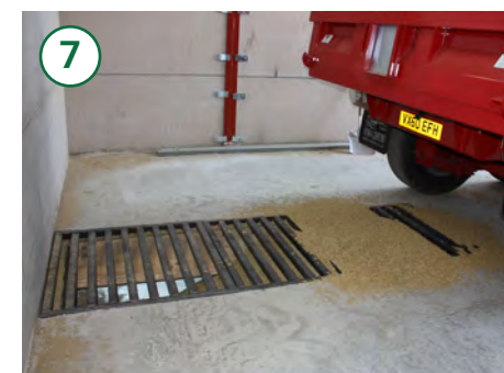
7 A sunken dryer with walled loading area to allow a substantial amount of grain to be piled up to feed the dryer. This prevents double handling as grain can be tipped into the loading area straight from the field rather than being tipped and moved with a handler. Beware not to place too much grain above the loading hopper without some sort of baffle to prevent the weight of grain crushing the hopper.
