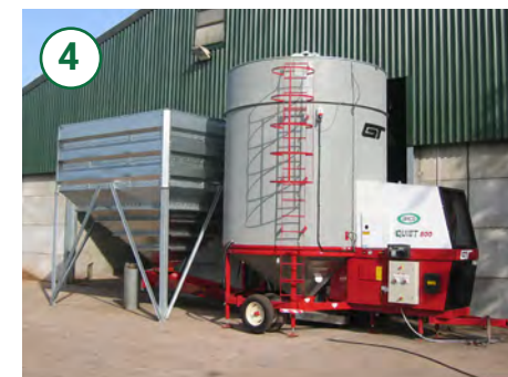
4 A buffer hopper ensures the dryer is filled as quickly as the loading hopper is able to take grain minimising downtime.
