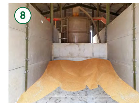
7 A sunken dryer with walled loading area to allow a substantial amount of grain to be piled up to feed the dryer. This prevents double handling as grain can be tipped into the loading area straight from the field rather than being tipped and moved with a handler. Beware not to place too much grain above the loading hopper without some sort of baffle to prevent the weight of grain crushing the hopper.
