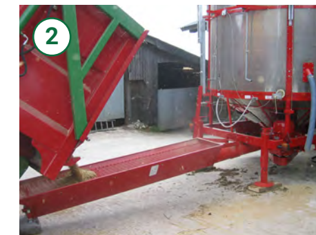
2 A 12 ton dryer takes the full capacity of the 12 ton trailers' grain chute to fill at maximum speed.
