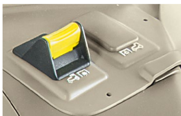
The cab-mounted Electro-Hydraulic PTO switch provides fingertip control of PTO engagement and disengagement.
