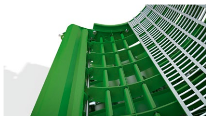
Once the locking bolts are released the concave section can be removed.
