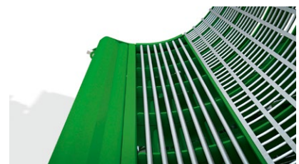
The new concave section is slotted into place and the locking nuts engaged.
