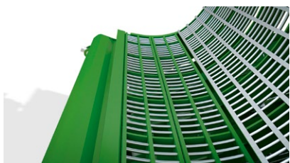
The front two sections of the separating concave are removable.
