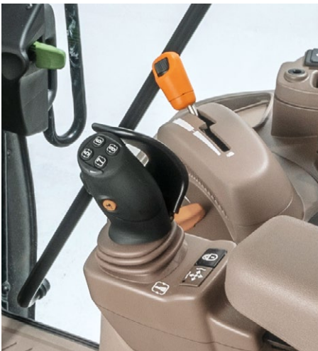
AutoPowr on the right-hand console
