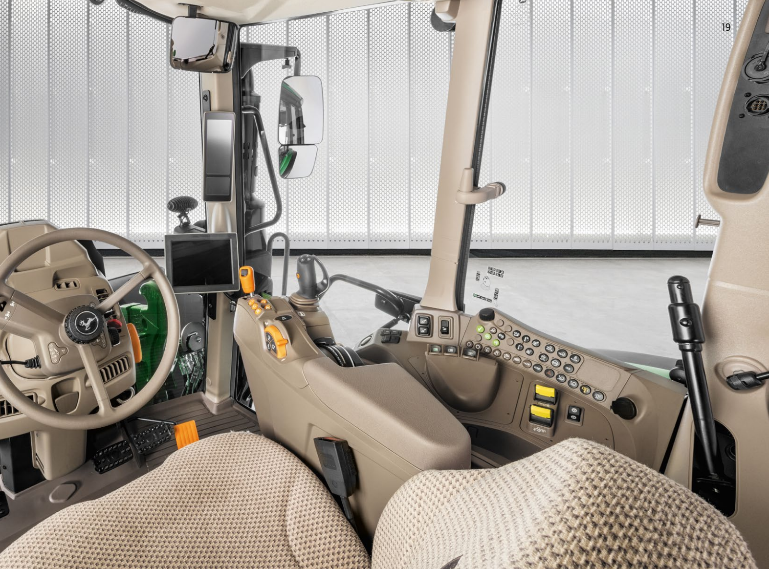
The intuitive interface to your 6M: The Corner Post Display in A-post and the new compact CommandARM.
