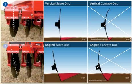
The end result is that the discs pull themselves into the ground more which assists penetration meaning more soil is inverted and residue incorporated. All this happens automatically and hydraulically as the depth of the discs is being altered by the tractor driver.
