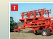
Rolls in transport position, wheels down
