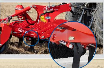
All models are available with hydraulic auto reset for extremely stony conditions. An individual hydraulic cylinder on each leg which is connected to a gas accumulator allows the leg to break back and reset if it comes into contact with an unmovable object.
