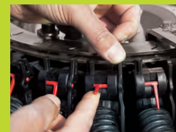
ADS head with management of seeded rows « on demand »
