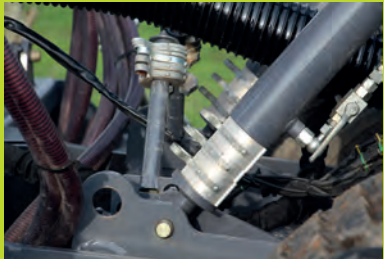
Centralised hydraulic setting of the drilling depth
