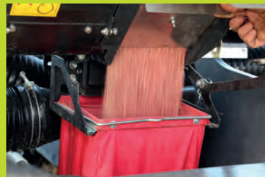
Emptying shutter Full emptying of the seed box
