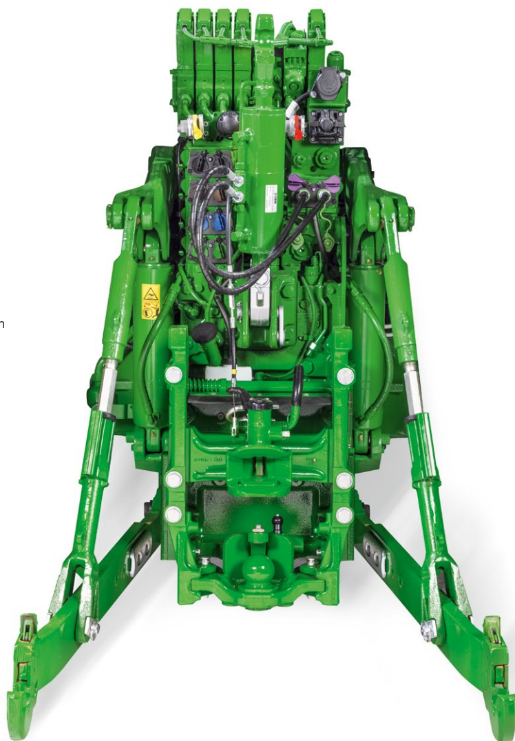
Automatic and mechanical wagon hitch with 38 mm ball-pin
