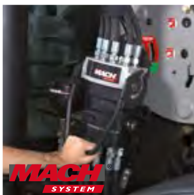
Instant electro-hydraulic connection tractor ↔ loader
