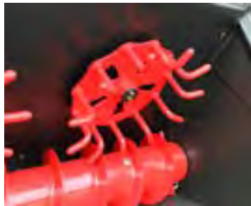
AGITATORS The feed agitators are mechanically driven by the auger screw. They break up any air pockets that might be created during distribution.
