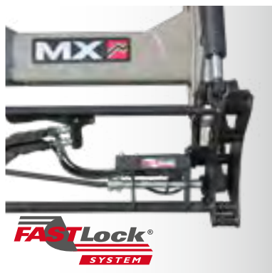
Automatic hitching/ unhitching of implements and hydraulic and electrical functions › page 48
