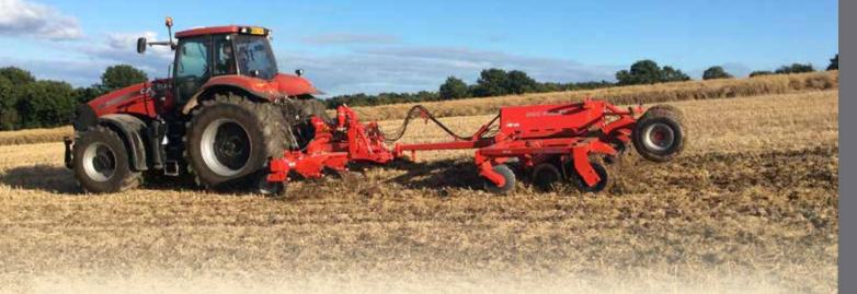
The Combi-Lift Pre-Cultivator fits directly to the tractor linkage and incorporates a rear clevis which can be used to pull a cultivator or drill. Furthermore, the machine can also be fitted with low-disturbance legs to enable light loosening of compaction without heave in mintill or direct drilling situations.
