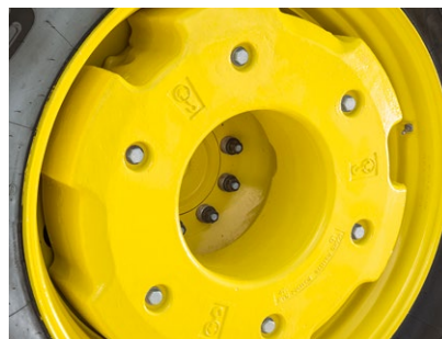
70 kg Starter Weight + 900 kg Heavy ballast for heavy pull with 42" or bigger rims.
