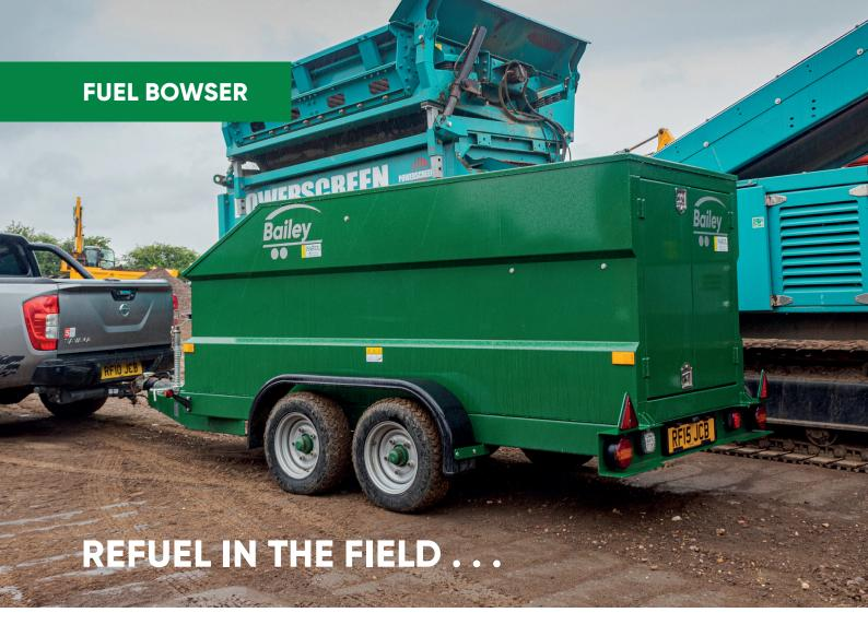
Our Fuel Bowser features a 2000 ltr fully bunded tank, with a 12v, 85 L/min pump positioned for easy access which is protected by a locking top panel. Also with lockable double back doors incorporating a 220 litre Adblue tank with pump and auto gun plus a storage shelf.
