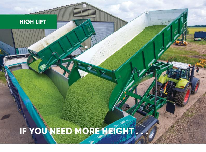
The 14 tonne High Lift trailer features a sprung drawbar and commercial axles mounted on heavyduty tandem springs.
