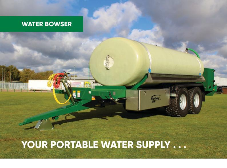
Our range of Water Bowser's features 4 capacity options of 12,000, 15,000, 16,500 and 18,000 litres. All models feature an elliptical, low centre of gravity translucent fibreglass tank.
