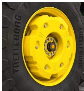
70 kg Starter Weight + 530 kg Compact weight in order to stay within 2.55 m.
