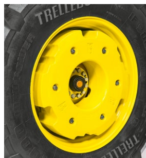
70 kg Starter Weight + 900 kg Heavy ballast for heavy pull with 42" or bigger rims.
