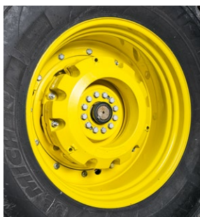
70 kg Starter Weight + 1x/2x 205 kg flexible ballasting fits all tyre sizes.
