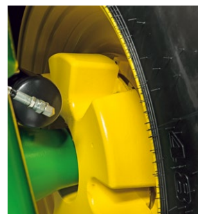
625 kg Inner weight, also possible with trailer brakes and additional oil out-take reservoir.
