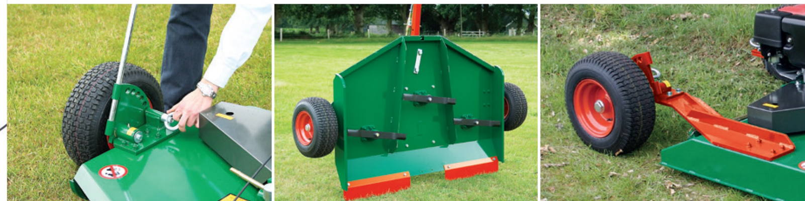
HEIGHT OF CUT IS SET BY REPOSITIONING THE WHEELS BY MEANS OF A SPRING LOADED PIN MECHANISM ON THE WHEEL BRACKETS
